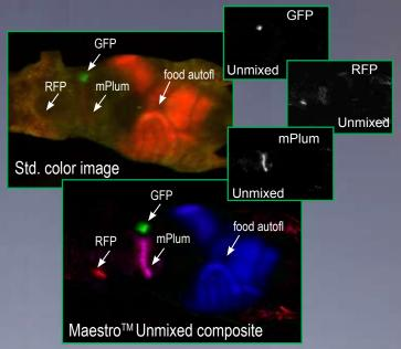
The Nuance™ (microscope mounted) and Maestro™ (in-vivo) fluorescence imaging systems cut through the fog of autofluorescence
